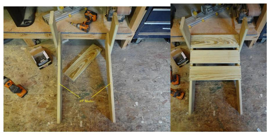
Make sure the bottom feet are 20 ½" apart on the inside (same as seat width). Use a clamp or temporary board fastened if necessary to hold to the correct width. Once that is achieved, mount the front stretcher across the front of the board at the base of the rear leg. Use 2 screws on each end, one into the front leg and one into the rear leg, pre-drill these beforehand.
