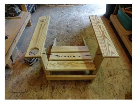
Mount the Back support, with the 20° beveled side facing up to the bottom of the arm rest, two screws on each side making sure the arm rest are spaced the same as the front part.
