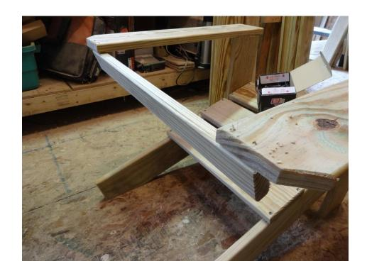
Fasten the arm support pieces with one screw on top and two on the inside of the front leg. Make sure it is in alignment with the back side of the front leg, leaving room for the cup holder.
