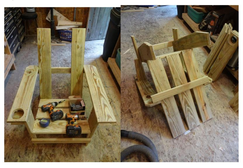
The chair is now assembled and should be sanded down to help eliminate any splinters and smooth out rough spots. At this point it could be stained if desired, but does not need anything since treated wood has been used. Seat cushions make a nice addition to the chair.
