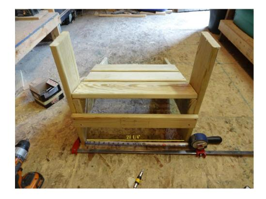
On both of the armrests, make a mark 1/2" in from the front; this is where to line up the front of the front leg. Pre-drill holes for the two screws into the front leg and one for arm support. Line up the inside of the front leg and inside of the arm and the  $\frac{1}{2}$ " mark and front of the front leg, then fasten only the front screw for each side.
