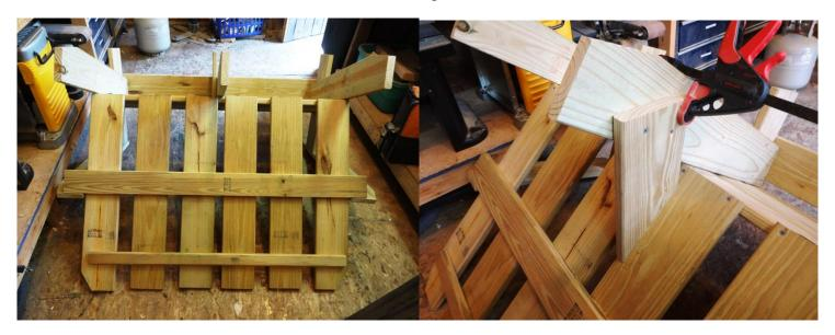
Flip the bench back upright. Pre-drill and fasten the arm supports under each arm rest. Use one screw going through the top and two going through the side. Once this is finished, give the bench a light sanding.
