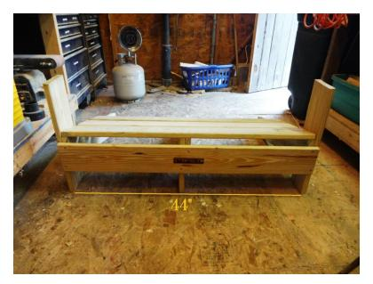
On both of the armrests, make a mark ½" from the front; this line will show where to position the front of the front leg for a little overhang. From the ½" mark draw a line 6" towards the back, 1" from the inside edge. This will show where the top of the front leg will be for pre-drilling. Fasten only the front screws at first. Measure the inside distances of the armrests front and back, making sure they are even and square with the chair.
