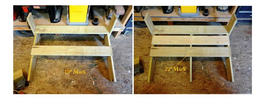
Making sure the bottom feet are 44" apart on the inside (same as seat width) and holding that, fasten the front stretcher board. Use two screws on each leg and pre-drill.
